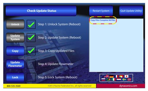
18. Press the **Update Flowmeter** button (Step 4: Update Flowmeter). A short process runs again indicated by text filling the text area.
