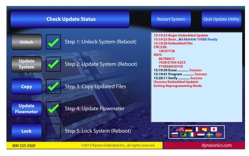
19. Press the *Lock* button and then remove the **USB Update Drive**.
