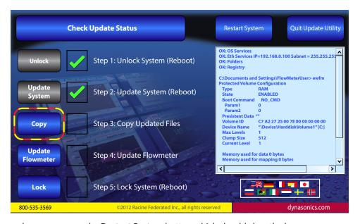
**NOTE:** If the process hangs-up, press the **Restart System** button which should clear the hang.
