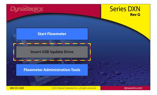
12. Insert the **USB Update Drive**. When the USB Update Drive containing the update is inserted the grayed out button changes to an active *Start Updater* button.
