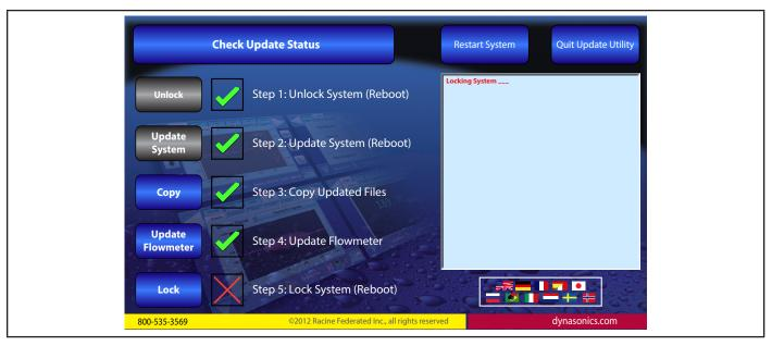
**NOTE:** See below for an additional instructions on clearing a lock-up with a hard reboot.
