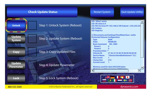
11. A small panel in the center of the screen asks if it is OK to reboot. Remove the **USB Update Drive** and then press the **OK** button.
